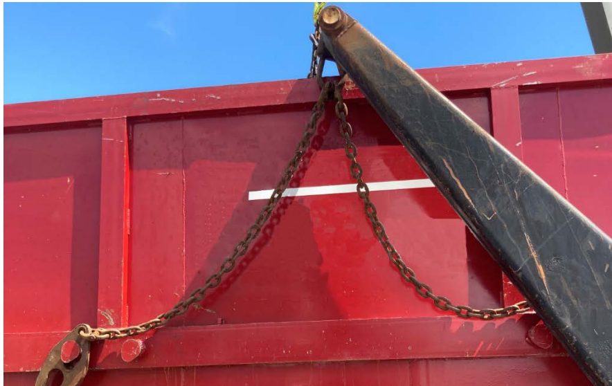
Rear lift chain may be loose during transit/roadside inspection
