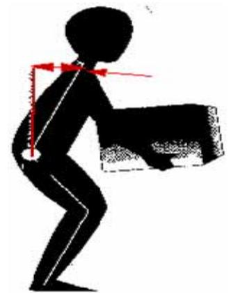
In many ways, your body works the same way as a material handler does when it is lifting. Your upper body is like lifting boom that pivots at your lower back. The longer the boom (shown with arrows in the picture above) the more strain on your back.
