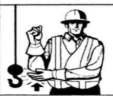
USE WHIPLINE. (Auxillary Hoist). Tap elbow with one hand; then use regular signals.
