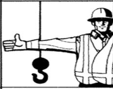
RAISE BOOM. Arm extended, fingers closed, thumb pointing upward.
