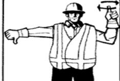
LOWER THE BOOM AND RAISE THE LOAD. Arm extended, fingers closed, thumb pointing downward, other arm with forearm vertical, forefinger pointing upward and rotate hand in horizontal circles.
