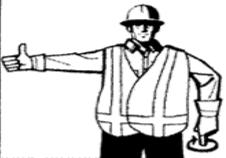
RAISE THE BOOM AND LOWER THE LOAD. Arm extended, fingers closed, thumb pointing upward, other arm bent slightly with forefinger pointing down and rotate hand in horizontal circles.
