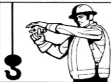
MOVE SLOWLY. Use one hand to give any motion signal and place other hand motionless in front of hand giving the motion signal. (Hoist slowly shown as example.)
