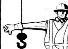
LOWER BOOM. Arm extended, fingers closed, thumb pointing downward.
