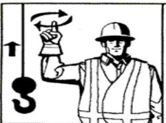
HOIST. With forearm vertical, forefinger pointing up, move hand in small horizontal circles.
