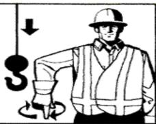
LOWER. With arm extended downward, forefinger pointing down, move hand in small horizontal circles.
