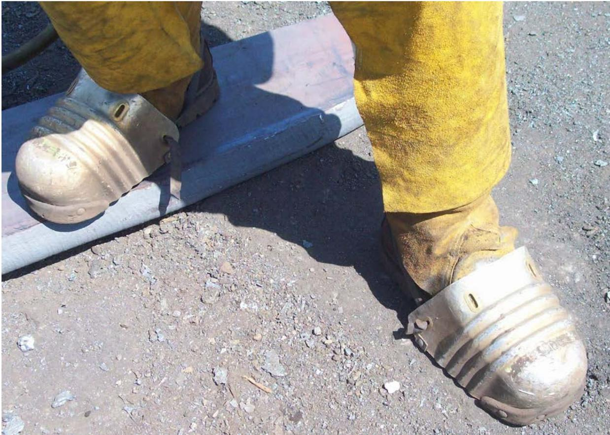
Removable steel toe caps can be worn outside regular steel toed boots and help save the leather boots from the rigors of hot slag dropping and burning while torching.
